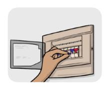
You can find out if a fuse has broken by checking a special box inside your home called a **fuse box**.
